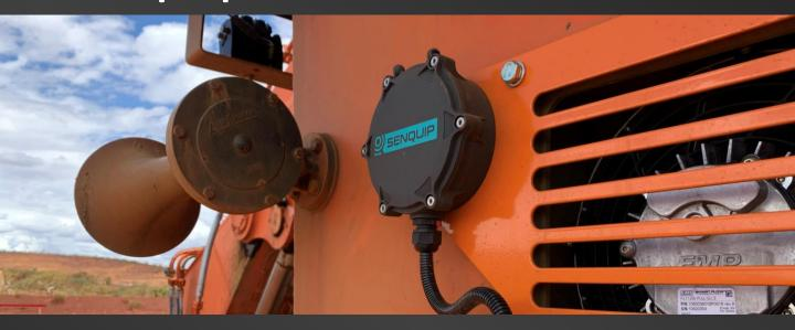
Senquip manufactures rugged, programmable telemetry devices that connect to industrial sensors and systems and send the data measured to the Senquip Portal or a server of your choice.
